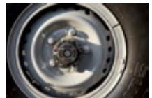
Auto and manual free-wheel hubs. Their only function is to save fuel on the open road. They must be engaged (manual) at the front wheels before the vehicle can be driven in four-wheel drive. Auto-free wheel hubs do not look like this as there is no manual lever or switch and are locked electrically when 4WD is engaged.
