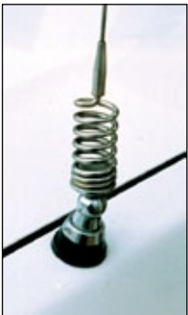
Top: Glass mount VHF. Middle: Body mounted HF with built-in single- frequency coil. Bottom: Body mount VHF.
