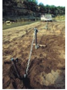
A recovery rig with multiple stakes. The more bits of chain, different sized shackles and lengths of strap you have, the easier it is to construct a complex rig.
