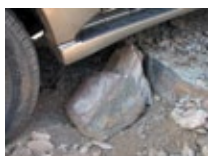
Packing rocks to make a descent easier. Bottom: Packing rocks to ease the angle of a rock ledge.
